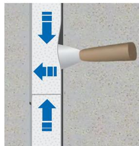
With vertical joints, start at the bottom and work your way up. Press the self-adhesive side of the tape (if necessary using a spatula) tightly against the joint edge. The ends of individual tapes must be butt-joined against each other without stretching the tape in the process.
