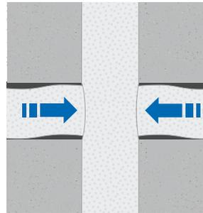
For cross- and T-joints we recommend to butt-join the horizontal tapes against the vertical. Please make sure to compress the tapes against each other.
